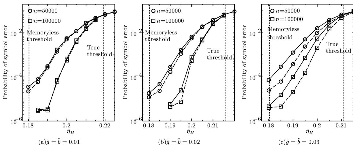
**Fig. 9** Experimental results for a  $(\lambda, \rho)$ -irregular LDPC code, where  $\hat{\theta} = (\hat{g} = 0.02, \hat{b} = 0.02, \hat{\eta}_G = 0.01, \hat{\eta}_B = 0.21)$  and  $\tilde{\eta}_G = 0.02$  are fixed. Solid lines represent the results for the GE-LDPC decoder which uses  $\hat{\theta}$ , and dashed lines represent the results for the ideal GE-LDPC decoder which uses  $\tilde{\theta}$ . Dotted lines represent the thresholds.
