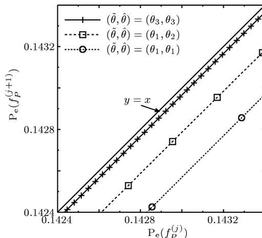
**Fig. 4** The EXIT chart of the proposed DE for the cases where the tuples  $(\tilde{\theta}, \hat{\theta})$  are set in  $(\theta_1, \theta_1)$ ,  $(\theta_1, \theta_2)$  and  $(\theta_3, \theta_3)$ , respectively, where  $\theta_1 = (g = 0.02, b = 0.02, \eta_G = 0.04, \eta_B = 0.37)$ ,  $\theta_2 = (g = 0.01, b = 0.01, \eta_G = 0.03, \eta_B = 0.39)$  and  $\theta_3 = (g = 0.02, b = 0.02, \eta_G = 0.04, \eta_B = 0.376)$ .
